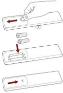
1. Slide the back cover to open the battery compartment of the remote control.
